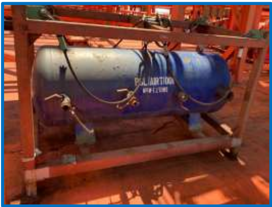
BA Air Accumulator Tank
