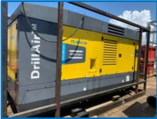
1,600-CFM Air Compressor
