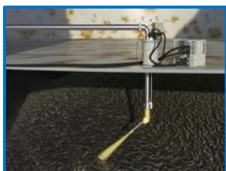
NOZZLES CLEAN TANK SIDES & TOP
