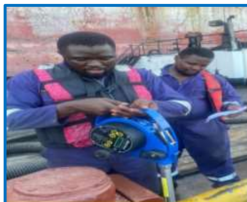
Oil / Water Interface Probe used to ID Depth of Oil, Water & Sludge in Tanks
