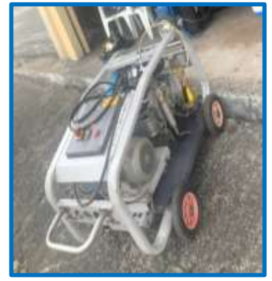
Breathing Air Generator
